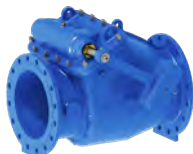
Series 41/36 Swing check valve Metal seated With lever and weight DN350-600 PN10/16 Ductile iron
