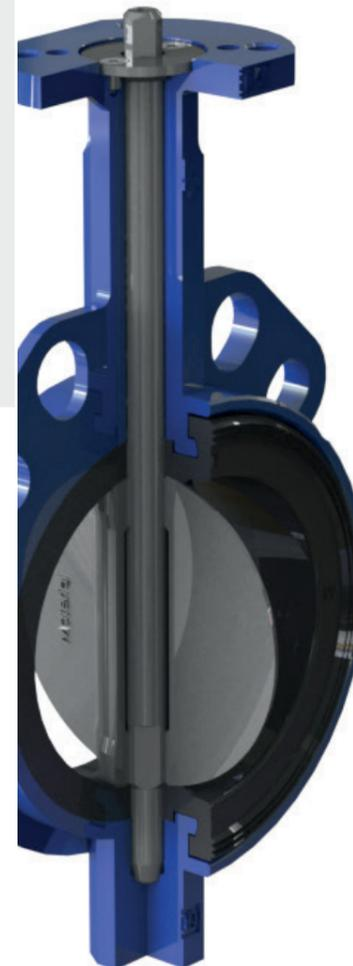
State-of-the-art anti-blow out shaft retention system with retaining collar and screws, which avoids the use of connecting pins between disc and shaft or other complicated systems
