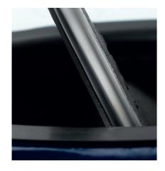
Profiled disc and unique AVK rubber ensure exceptional durability The unique AVK rubber compound has an excellent ability to regain shape after compression, and this ability combined with the profiled disc secure tightness even after thousands of operation cycles.
