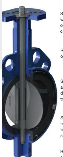
State-of-the-art anti-blow out shaft retention system with retaining collar and screws, which avoids the use of connecting pins between disc and shaft or other complicated systems
