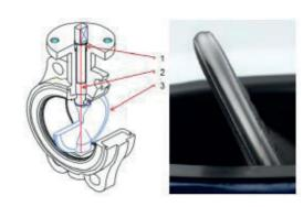
Compared to Double Eccentric Butterfly Valve which requires a higher operating torque values. This means a bigger gearbox/ actuator which will impact on the total cost of the valve and actuator and also increasing the operating cost on the end user as more power will be consumed.
