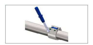
A Repico® coupling weighs less than half of 2 flanges. Pipe supports can be lighter, transport cost is lower and for some applications the net weight for cargo increases.
