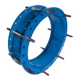
AVK dismantling joints provide easy installation and disassembly of flanged pipework and equipment and compensate for axial displacement of the pipe during installation and dismantling. The range is available in DN50-2400 in PN10, PN16, PN25, PN 40 and PN 60 or ANSI CL150, CL300, CL600 and CL900.
