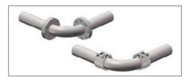
A Repico<sup>®</sup> coupling is smaller than a flange. You require less storage space, less transportation capacity, less space to install the pipe or get more pipes close together in a smaller space.
