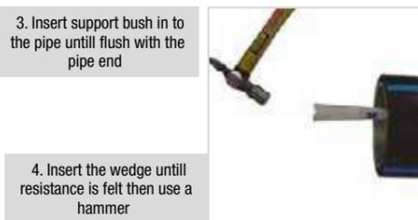
4. Insert the wedge until resistance is felt then use a hammer
