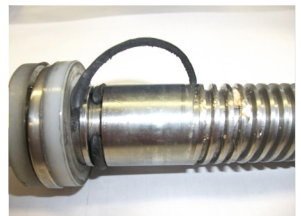
Damaged spindle thread and O-ring
