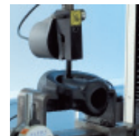
A thin layer of rubber must remain after the peeling test.
