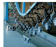
The double bonding process prevents creeping corrosion.
