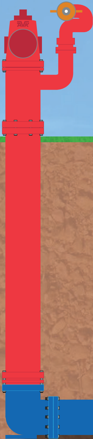
AVK dry barrel hydrant with monitor
